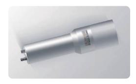
ENAI-D76H76VD01 scintillator detector is composed of a 3-inch Nal scintillator crystal, photomultiplier tube and voltage divider. Due to its high detection efficiency, good energy resolution, flexible matching, stable performance and easy to use, it is widely used in the fields of energy spectrum measurement analysis, building materials, food and other radioactive level analysis.
