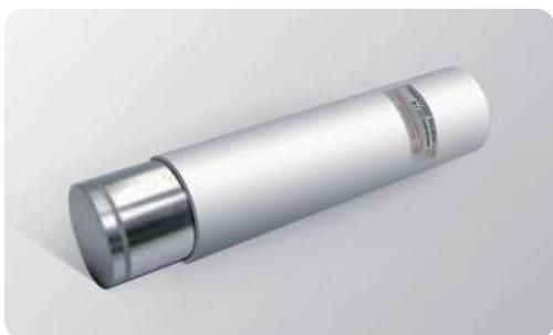
The ENAI-D50H50DHP01 scintillator detector is a highly integrated detector composed of a 2-inch NaI scintillator, photomultiplier tube, voltage divider, high-voltage module, and preamplifier. It can be used for gamma ray energy spectrum measurement, directly output negative polarity signal. Due to its high detection efficiency, good energy resolution, and stable performance, it is widely used in energy spectrum measurement analysis, densitometry, coal ash analysis and other fields.
