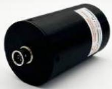
The ELBC-D50H50SIPM01 spectroscopic detector is a highly integrated detector containing a 2-inch  $\text{LaBr}_3(\text{Ce})$ , silicon photomultiplier (SiPM), summing circuit, preamplifier circuit, and temperature measurement circuit. It features excellent energy resolution, simple operation, compact size, and high reliability. It is widely used in industrial detection, radiological medicine, radiation detection, and other fields.
