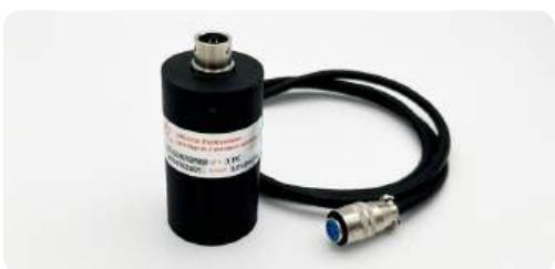
The ELBC-D25H25SIPM01 spectroscopic detector is a highly integrated detector containing a 1-inch  $\text{LaBr}_3(\text{Ce})$ , silicon photomultiplier (SiPM), summing circuit, preamplifier circuit, and temperature measurement circuit . It features excellent energy resolution, simple operation, compact size, and high reliability. It is widely used in industrial detection, radiological medicine, radiation detection, and other fields.
