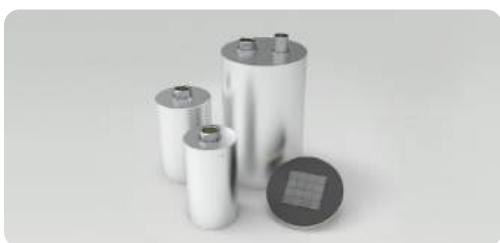
The ECB-D38H38SIPM01 spectroscopic detector is a highly integrated detector containing a 1.5-inch CeBr<sub>3</sub>, silicon photomultiplier (SiPM), summing circuit, preamplifier circuit, and temperature measurement circuit. It features excellent energy resolution, simple operation, compact size, and high reliability. It is widely used in industrial detection, radiological medicine, radiation detection, and other fields.
