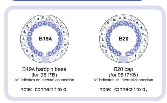
Our range of B19A sockets is available to suit the hardpin base. Our range of B20 sockets is available to suit the B20 cap. Both socket ranges include versions with or without a mounting flange, and versions with contacts for mounting directly onto printed circuit boards.
