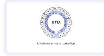
Our range of B19A sockets, available for this series, includes versions with or without a mounting flange, and versions with contacts for mounting directly onto printed circuit boards.
