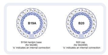
Our range of B19A sockets is available to suit the B19A hardpin base. Our range of B20 sockets is available to suit the B20 cap. Both socket ranges include versions with or without a mounting flange, and versions with contacts for mounting directly onto printed circuit boards.
