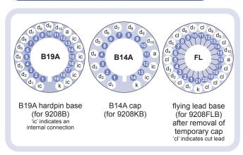
Our range of B19A sockets is available to suit the B19A hardpin base. Our range of B14A sockets is available to suit the temporary B14A cap when the flying lead base variant is selected. Both socket ranges include versions with or without a mounting flange, and with contacts for mounting directly onto printed circuit boards.
