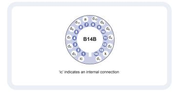
Our range of B14B sockets, available for this series, includes versions with or without a mounting flange, and versions with contacts for mounting directly onto printed circuit boards.
