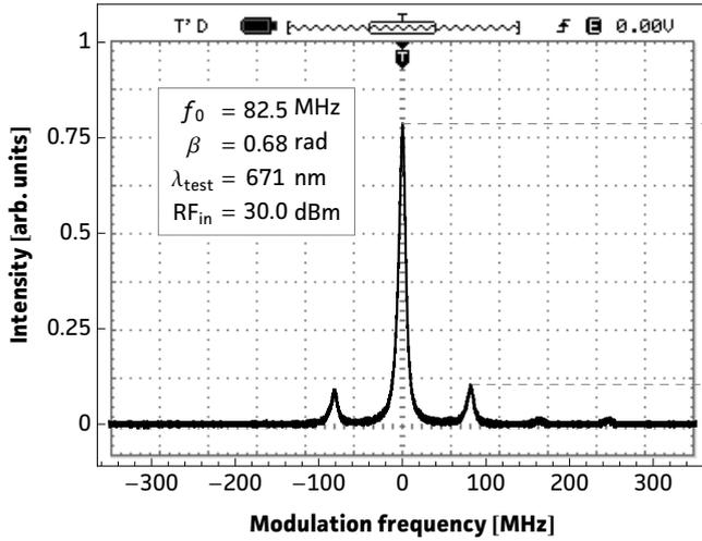
**Fig. 2: Carrier/sideband ratio**
